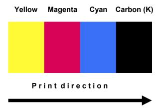
For special needs, we are also offering color ribbons with an additional K field. This is a useful option if e.g. a customer needs to print the front of a card in YMCK while on the back of the card has to be printed only some text information in K. The CMYKK ribbon enables this process without the use of a double patch of YMCK and is very cost saving.
